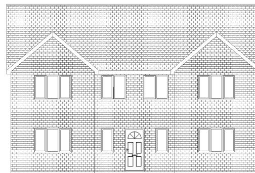
Note: You can add basic hatching to your drawing using the processes described above, but pressing the **Hatch** button rather than the **Hatch Patterning** button after selecting the polyline.
