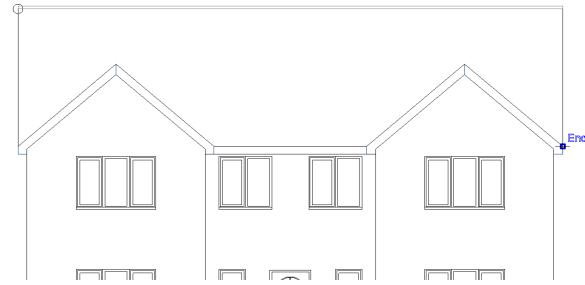
15. Continue clicking around the roof in a clockwise direction on each of the 'End' corner points until you get to the bottom left hand corner of the roof.
